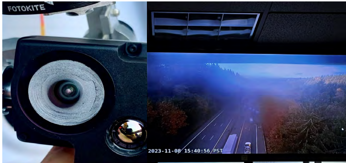
Figure 7: Condensation at the Fotokite camera lens
