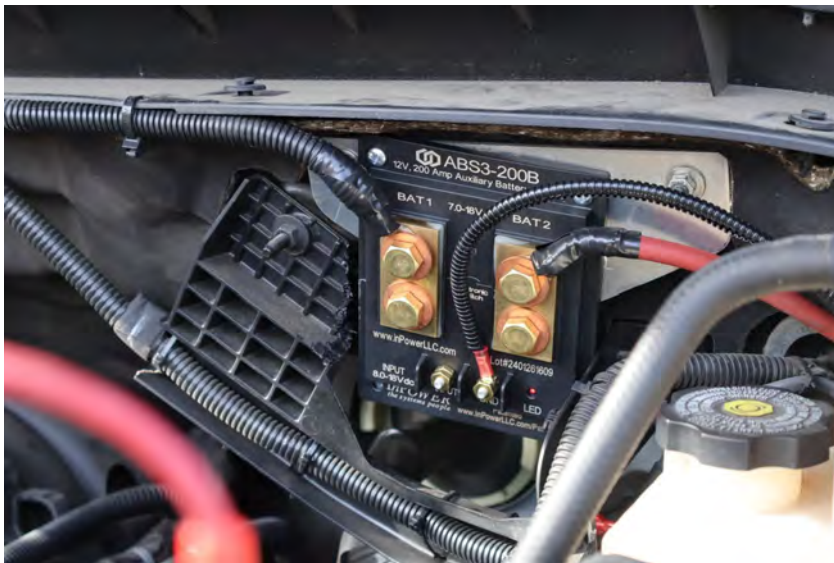
Figure 12: Malfunctioned auxiliary battery switch
