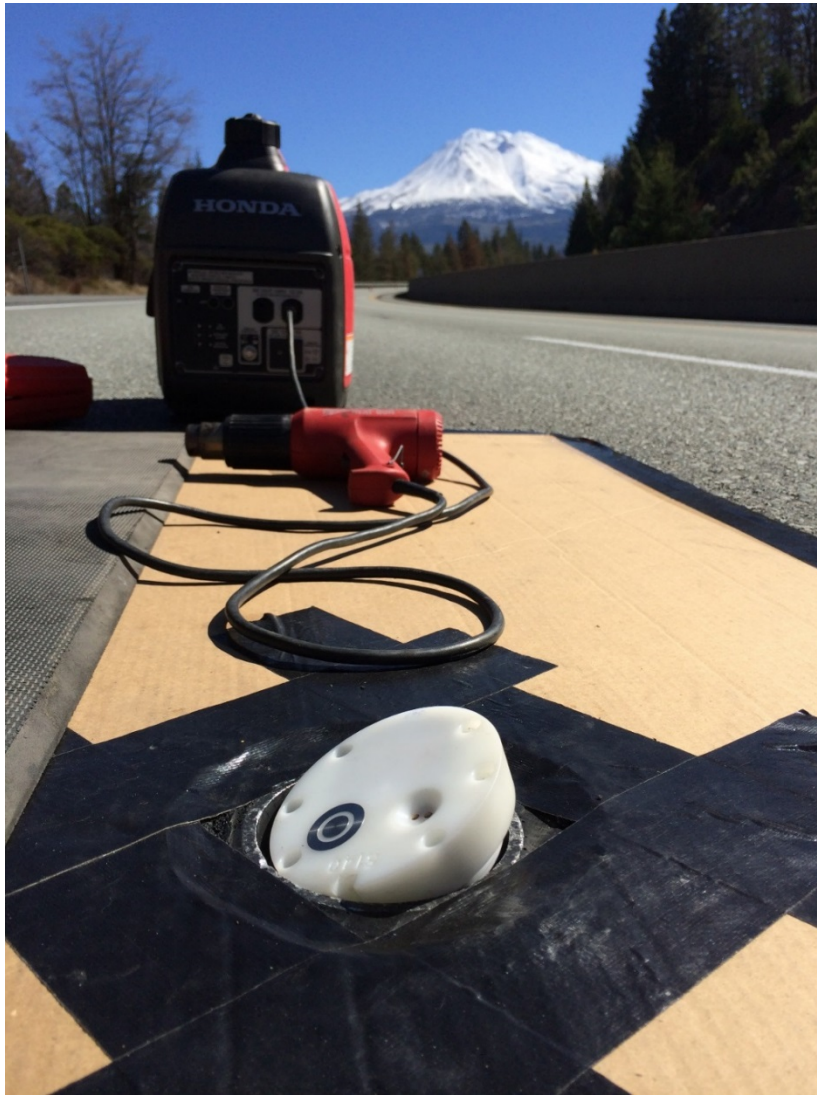
Lufft RSS are removable from a housing.
