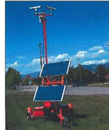
Solar power allows traffic sensors to be deployed anywhere-anytime needed.
