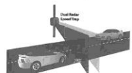
Dual Radar determines vehicle speed by measuring the delay from radar return to the road. This also determines vehicle direction.
